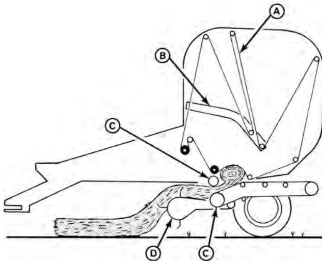
FIGURE 1. International Harvester 241 Bigroll Balers: (A) Bale Forming Belts, (B) Tensioning Arm, (C) Compression Rollers, (D) Pickup.
