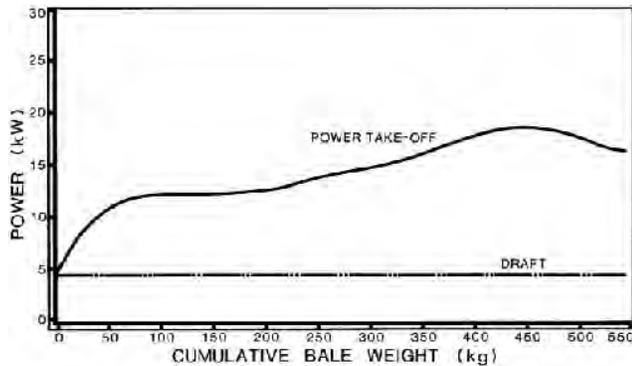
FIGURE 5. Power Consumption During Bale Formation in Alfalfa.
