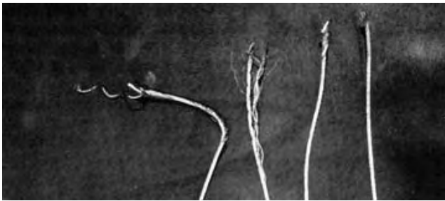
FIGURE 10. Damaged Bale Forming Cables.
