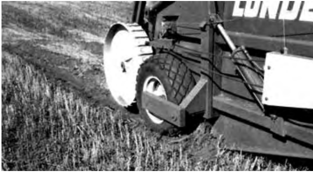
FIGURE 9. Skidding of the Drive Wheels on Rough, Irregular Ground Surfaces.
