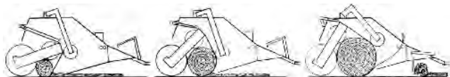
FIGURE 11. Stages of Bale Formation: (Left) Bale Core, (Centre) Half-Completed Bale, (Right) Completed Bale with Second Bale Starter Lowered for Twine Wrapping.
