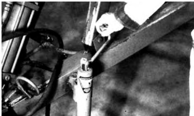
FIGURE 15. Hitch Jack Handle Interference.
