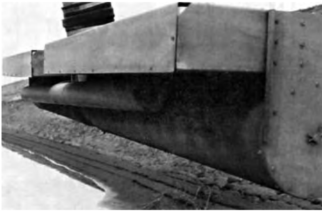
FIGURE 12. Intake Pipe Suction Screen.
