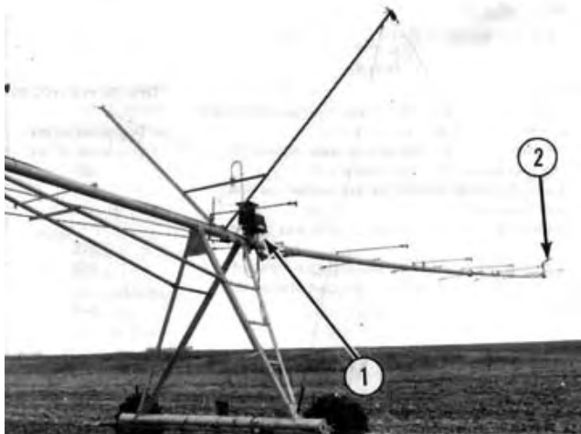
FIGURE 21. Booster Pump (1) and End Gun (2).
