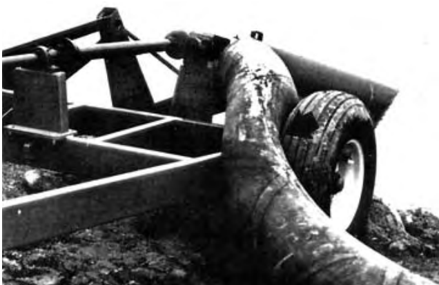
FIGURE 5. Improper Discharge Hose Placement Resulting in a Discharge Restriction.
