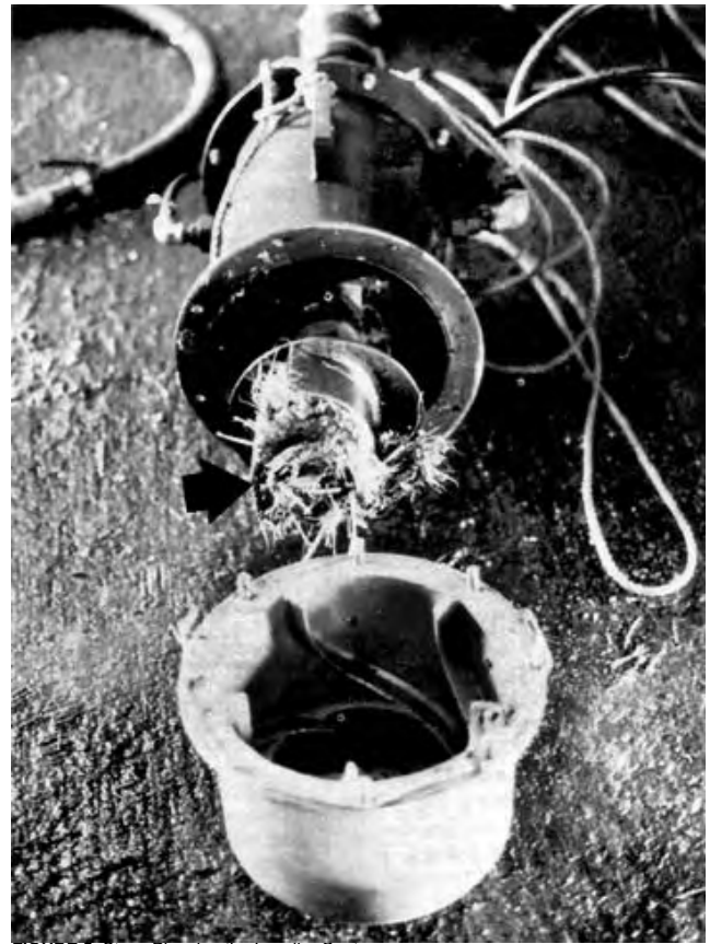
FIGURE 5. Straw Plugging the Impeller Centre.
