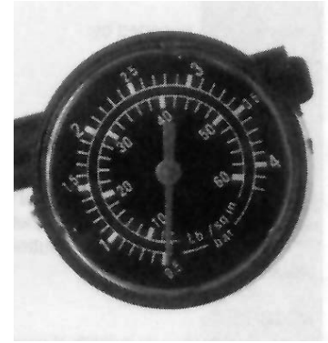
Figure 2. Gauge pressure indicator.
