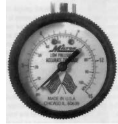
Figure 2. Gauge pressure indicator.
