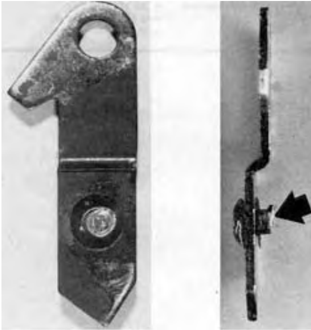
FIGURE 6. Interference between Pump Handle and Rivet.
