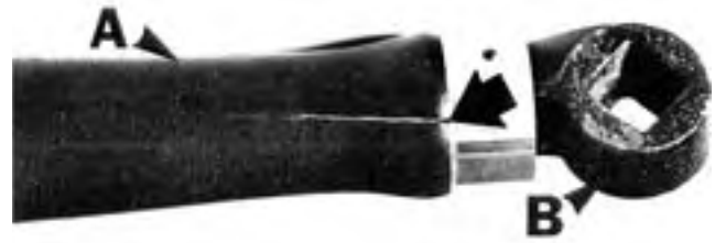
FIGURE 4. Split Pump Handle: (A) Pump Handle, (Bi Cast Iron Adaptor.
