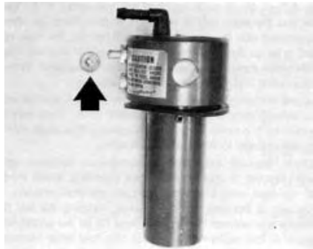
FIGURE 7. Broken Control Valve Knob.
