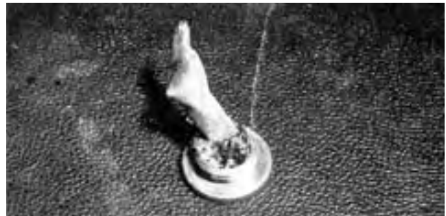
FIGURE 4. Plugged Outlet Nozzle Strainer.
