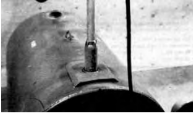
FIGURE 4. Impeller Housing Too Large for 50 mm Fuel Supply Tank Opening.
