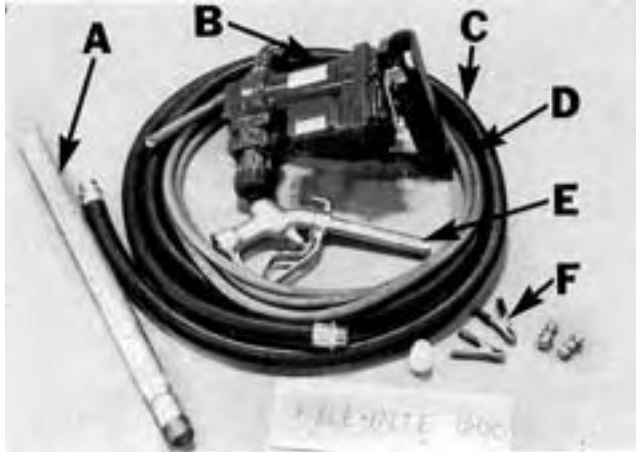
FIGURE 1. Fill-Rite Model 1210 Fuel Transfer Pump: (A) Telescoping Suction Pipe, (B) Pump Body, (C) Outlet Hose, (D) Battery Cable, (E) Nozzle, (F) Alligator Clamps.
