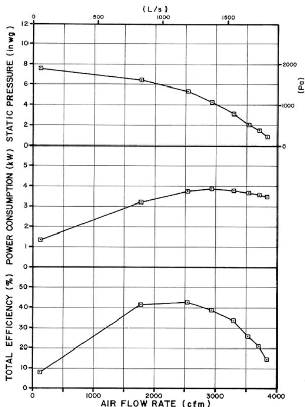
FIGURE 3. Westeel Model WVA-18-3-1 Fan Performance Curves.
