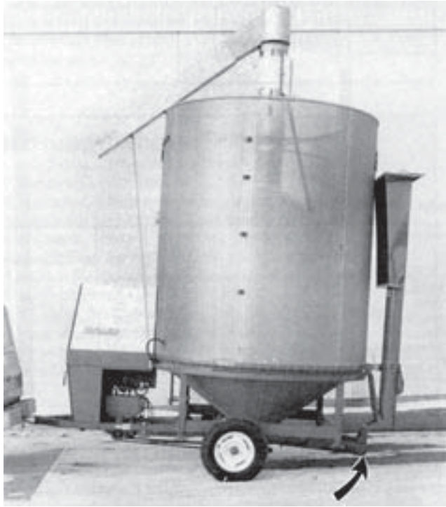
FIGURE 2. Minimal Ground Clearance on Uneven Terrain.
