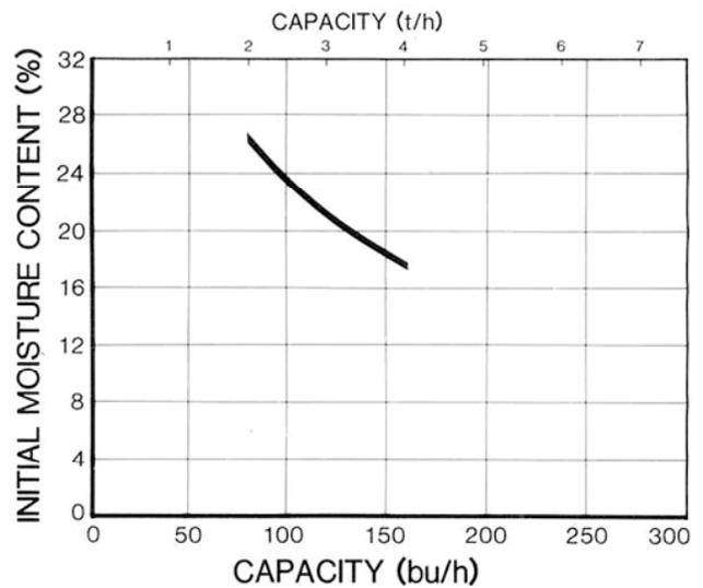
FIGURE 14. Drying Capacity in Corn (Hybrid 3996).
