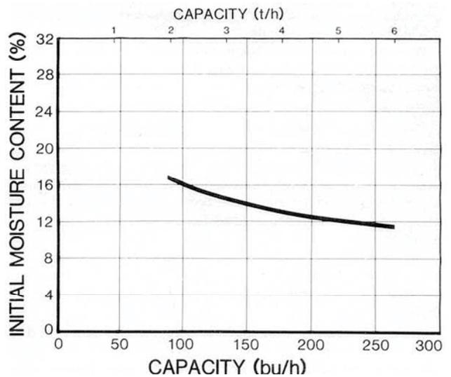
FIGURE 13. Drying Capacity in Rapeseed.
