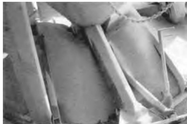
FIGURE 10. Fines Accumulated Under the Dryer.
