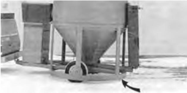
FIGURE 2. Minimal Ground Clearance on Uneven Terrain.
