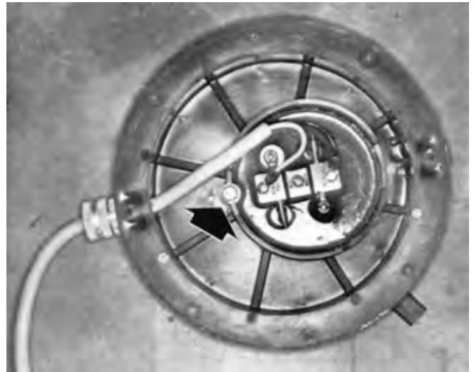
FIGURE 7. Grain Pressure Switch Sensitivity Adjustment.
