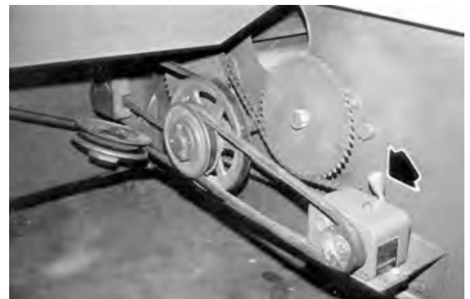
FIGURE 8. Metering Roll Speed Adjustment.
