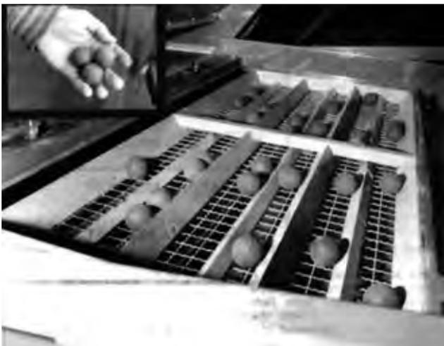
FIGURE 3. Screen Frame (Hard Rubber Balls Shown in Inset).
