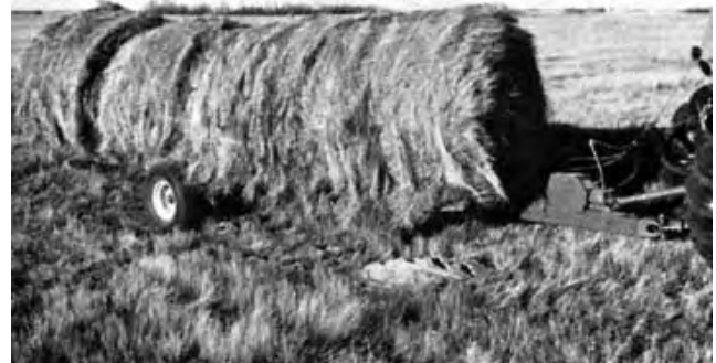
Figure 5. New Holland 85 Fully Loaded in Transport Position.
