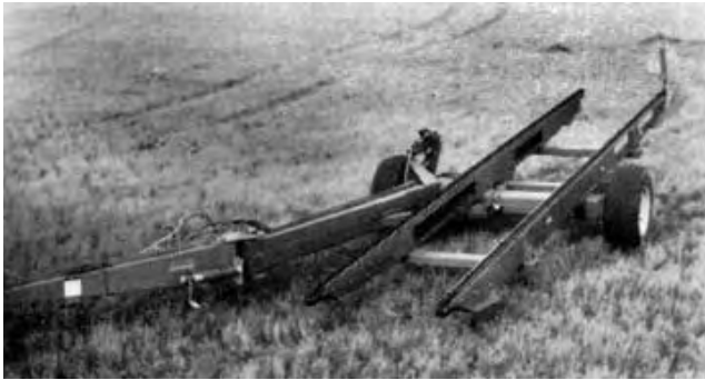
Figure 2. Hesston 5200 in Loading Position.
